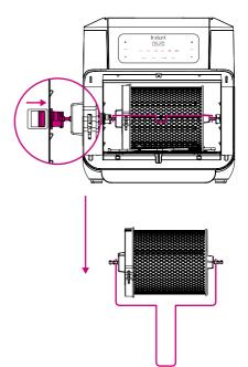
Rotisserie spit, forks, and basket will be hot during and after cooking. Always use the rotisserie lift to remove rotisserie accessories, and exercise extreme caution when removing hot accessories from the cooking chamber. Always use Instant Pot® Mini Mitts or oven mitts when disassembling hot rotisserie accessories.
