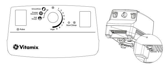
On/Off Switch (I)/(O): The switch is located on the front left side of the machine below the control
