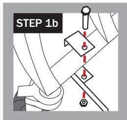
Slide Gas Tank Caddy under Cart, so top bracket piece rests on cart frame and is lined up with bolt hole on bottom of Gas Tank Caddy. Reinsert bolt into frame and tighten together with nut (Step 1b). Use the provided wrench to tighten all connections.
