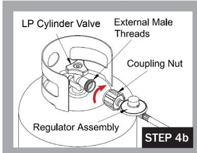
Make sure the cylinder valve is closed (turn valve clockwise until tight). Inspect valve connections, port, hose and regulator assembly for any damage or debris. Remove any debris.
