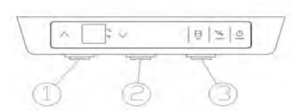
Light switches are under the control panel to control the lights turn on/off:
