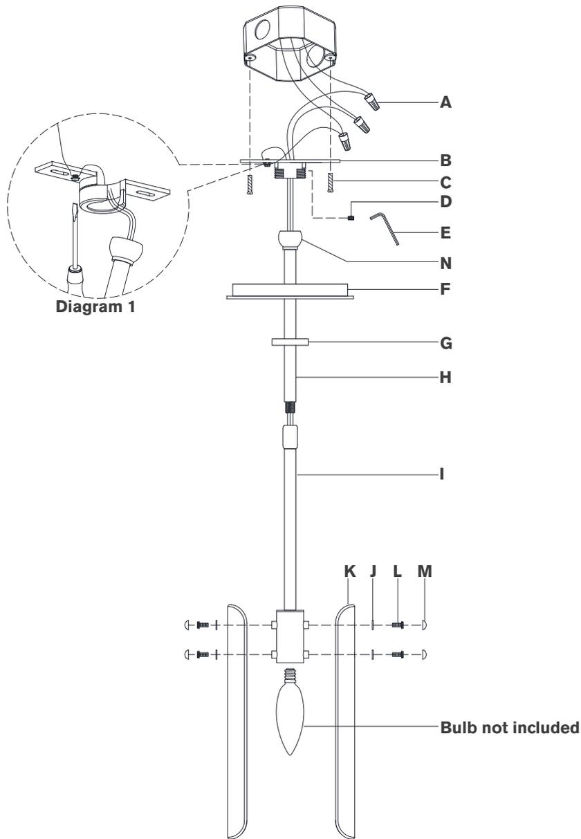
10. Connect fixture neutral wire (white) to the supply neutral wire (usually white) using wire nut **(A)**.
