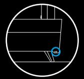
There is also the option to loosen off the door hinges. Use the supplied allen key to loosen the hinges on the sides of Uuni Pro as shown in adjacent diagram. Once loose, you can slide the door hinges forward slightly before securing them again: This gives the door more room for expansion and will make it easier to add and remove from Pro.
