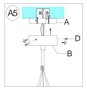
5. With the help of another person to hold the weight of the Chandelier, Raise the Canopy (B) up over the Mounting Plate (A), aligning the 3 holes from the Mounting Plate (A) with the 3 holes on sides of the Canopy (B). Insert the 3 Canopy Screws (D) and tighten each screw with a screwdriver until secure.
