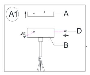
Separate the Mounting Plate (A) from Canopy (B) by removing the Canopy Screw (D). Do not discard Canopy Screws (D) as these will be used later.
