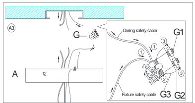
3. Wrap the safety steel wire from the light fixture and the safety steel wire from the ceiling onto the safety Cable (G), Tighten the cap nuts (G2) to secure the safety wires
