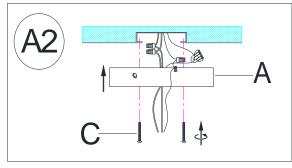
2. Insert the J-box wires through the center opening of the Mounting Plate (A) Attach the Mounting Plate (A) to the outlet box using the two J-Box Mounting Screws (C). Tighten each screw clockwise until the Mounting Plate (A) is firmly secured to the J-Box.
