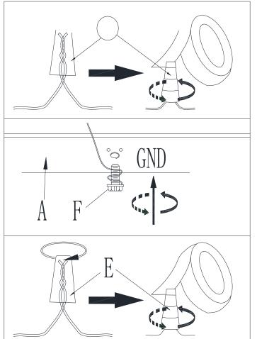
Connect the GROUND FIXTURE WIRE to the GROUND J-BOX WIRE using the Plastic Wire Nut Connector (E) and wrap the connection with electrical tape. Be sure that no wire strands are exposed.
