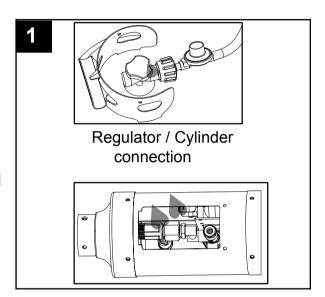
If NO bubbles appear at any connection, the connections are secure.
