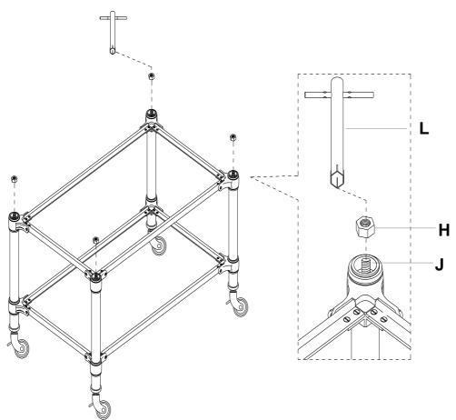
6. Hand screw Finials (A) onto top of the Threaded Rods (J) as shown.
