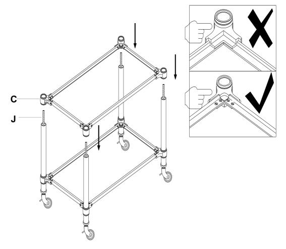
4. Slide Washer (B) over the Threaded Rods (J) as shown.
