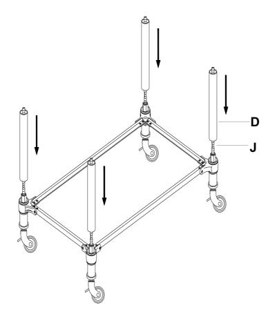
3. Slide Metal Frame (C) over the Threaded Rods (J) as shown.
