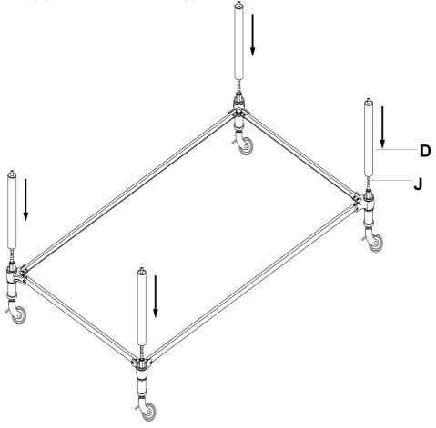
Date: 14-Apr-16 Rev: 3. Slide Metal Frame (C) over the Threaded Rods (J) as shown.
