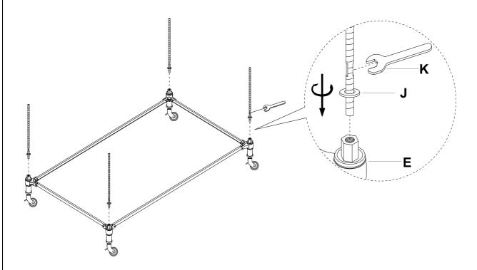
2. Slide four Poles (D) over the Threaded rods (J) as shown.
