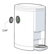
**WARNING:** Be sure to unplug your Spinn before removing the cap to avoid injury from moving parts.
