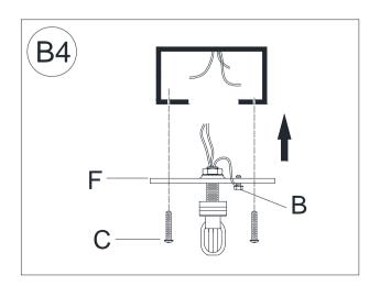
With the help of another person to hold the weight of lighting fixture, attach the Mounting Plate (F) onto the junction box using two Mounting Screws (C). Tighten each screw clockwise with a screwdriver.
