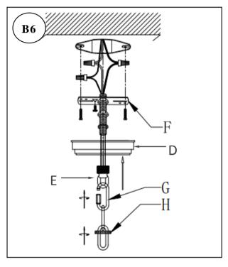
Slide the Canopy (D) upward along the chain until the upper rim of the canopy pressed gently against the ceiling surface. Position the Canopy Nut (H) against the Hanging Loop (E) and rotate the nut clockwise to engage it with the threaded portion of the Hanging Loop (E) until secure. Do not over tighten this nut.
