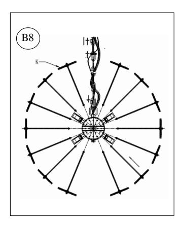
Insert the Metal Rods with Glass Dish (K) into the threaded holes that located around the fixture ball. Rotate each Metal Rods with Glass Dish (K) clockwise until tight.
