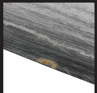
Blade discoloration can be polished off. Desirable patina protects the carbon steel of a Shun Blue
