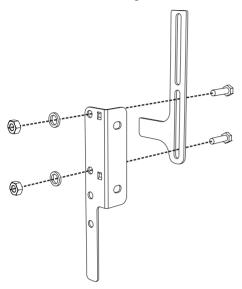
2. Align the base of the hook on the fastening bracket with the base of the slot on the wall fastening plate.
