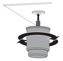
The appliance must sit level on the floor to ensure stability.
