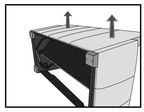
**5.** With the four bolts removed (from the previous step), the back can now be lifted away from the sleeper and set aside.
