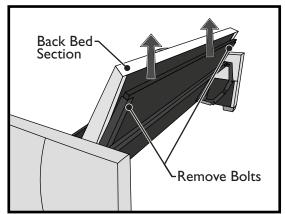
6. Remove (4) four bolts on each side of the comfort sleeper that secure the back bed section to the mechanism. Start from the bottom, leaving a single top bolt on each side. Hold the back bed section while removing the last two bolts. Set the back bed section aside.
