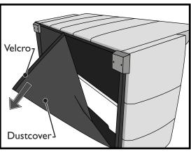
**3.** Roll the comfort sleeper forward, as shown. Open the dustcover on the bottom by pulling to release the velcro holding it closed.
