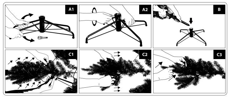
• Assemble the tree stand by pulling apart the legs of the stand so that they are X-shaped. Match the hole of the plastic flange with the pre-drilled hole in the stand. Screw the eyebolt through the hole in the stand, making sure it does not protrude into the center of the stand so that the tree trunk can be inserted easily into the stand. (See Figure A1 and A2)
