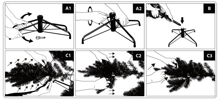
• Assemble the tree stand by pulling apart the legs of the stand so that they are X-shaped. Match the hole of the plastic flange with the pre-drilled hole in the stand. Screw the eyebolt through the hole in the stand, making sure it does not protrude into the center of the stand so that the tree trunk can be inserted easily into the stand. (See Figure A1 and A2)
