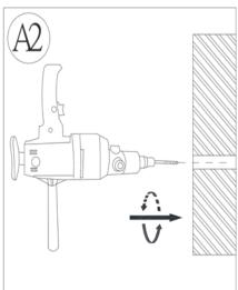
Using a drill with a properly sized drill bit (just big enough to make a hole for plastic anchor assemblies (A)), drill a hole in the ceiling at each of the two locations marked for plastic anchors (A).
