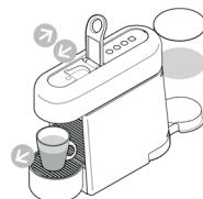
⑤ Remove the cup. Lift and close the lever to eject the capsule into the used capsule container.
