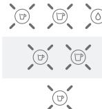
Espresso, Lungo, Hot water blinking: Hard
