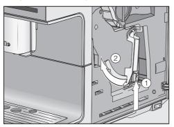
■ Press and hold the button under the brew unit handle ① and, while doing so, turn the handle to the left ②.
