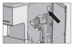
**Tip:** The milk pipework can be stored behind the service panel when not in use.
