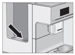
The water container filter is located under the water container.
