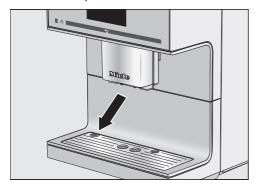
Remove the protective film from the drip tray cover and place it into the lower panel.
