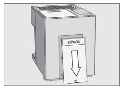
■ Slide the cover at the back of the coffee machine downwards.
