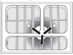
■ Clean the fill level sensors (see illustration) with a soft, dry cloth.
