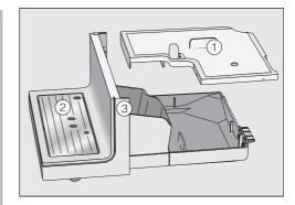
■ Remove the drip tray cover ①, the drip tray ②, and the lower panel ③.
