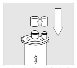
Seal the descaling cartridge with the cap.
