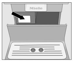
The password of your coffee machine is the serial number located on the data plate.
