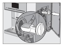
Fill the coffee scoop with ready ground coffee. Push the ground coffee drawer horizontally into the ground coffee chute.
