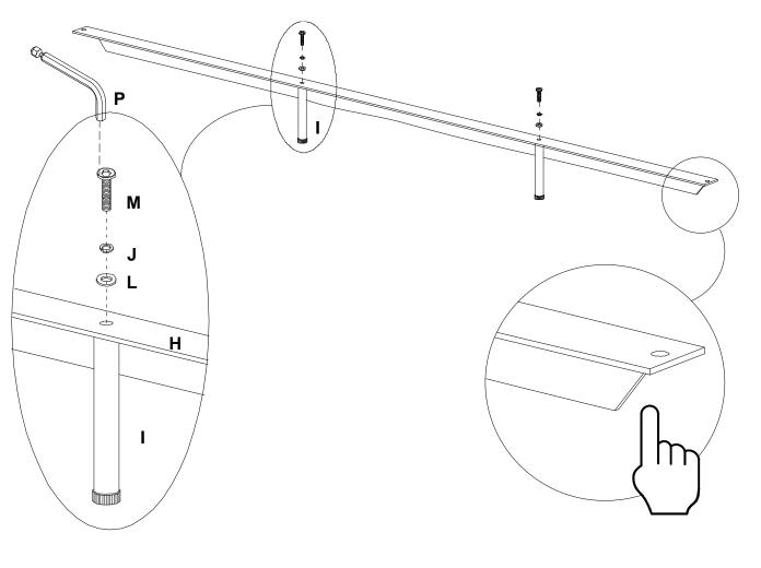
6. Attach the Slat (H) to Side Rail (E) by using Bolt (M), Spring Washer (J), Flat Washer (L) and Nut (N), tighten with Allen Wrench (P) and Open Wrench (Q).
