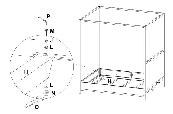
Finally, fully tighten all bolts with the provided Wrench, assembly is complete!
