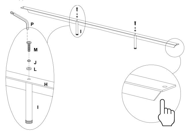
Date: 16-May-16 Rev: 6. Attach the Slat (H) to Side Rail (E) by using Bolt (M), Spring Washer (J), Flat Washer (L) and Nut (N), tighten with Allen Wrench (P) and Open Wrench (Q).
