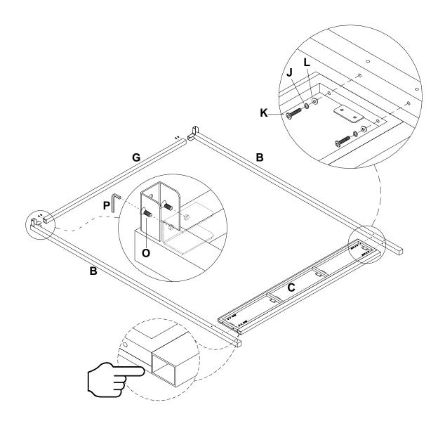
Date: 16-May-16 Rev: 2. Attach Post (A) to Short Stretcher (G) and Headboard (D) as shown, secure the Short Stretcher (G) by using Bolt (O), secure the Headboard (D) by using Bolt (K), Spring Washer (J) and Flat Washer (L), tighten with Allen Wrench (P).
