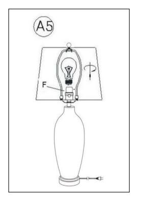
Insert the specified light bulb into the Socket (F). DO NOT EXCEED THE SPECIFIED WATTAGE.
