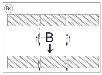
Insert the Stud Anchors (B) into each of the 4 ceiling holes.
