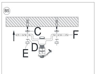
1. Place Cross Plate (F) to ceiling outlet box, letting bottom threaded section of Stud Anchors (B) pass through the inner holes of Cross Plate (F) and secure with Nuts (E) .Note: Place Flat Washer (C) in between the Stud Anchors (B) and the Cross Plate (F); Place Spring Washer (D) in between with Cross Plate (F) and Nuts (E).
