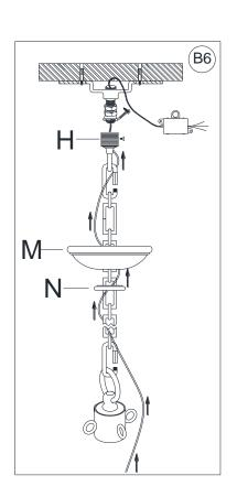
Weave the fixtures power cord through every other loop to the top of Chain (L), and then through the Hanging Loop (H) and Nipple (I), and come out from the center hole of the Cross Plate (F).
