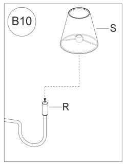
Attach center cup of shade (S) onto top of the candle cover (R).
