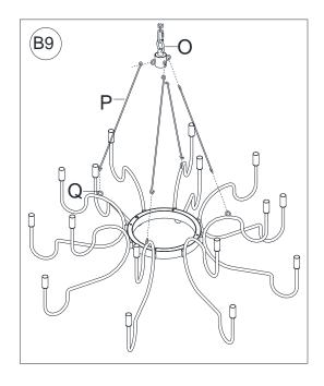
Hook the hooks (P) onto the fixture loop (O) and rings (Q) on light fixture.
