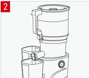
2 Press the locking tab down until you hear a click to completely secure the auto hopper lid. Place the juice cup and pulp cup under their corresponding spouts.
