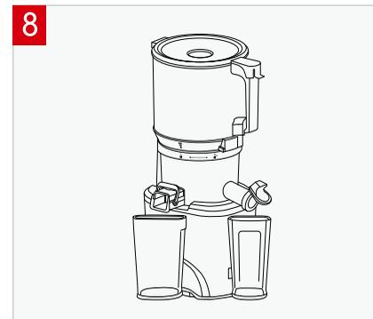
Place the pulp cup under the pulp spout and the juice cup under the juice spout as shown in the illustration.
