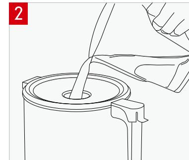
Pour water through the auto hopper opening and let the juicer operate for 30 seconds.
