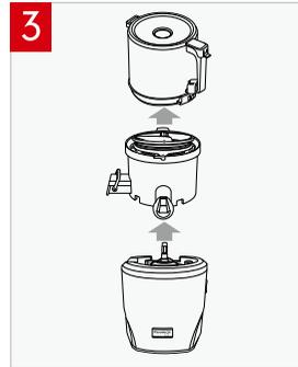
Lift the auto hopper and juicing chamber in sequence and separate them from the base.
