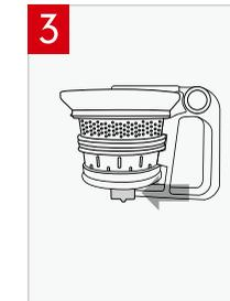
Slide the lock tab towards the tip of the base until it firmly locks into position.
