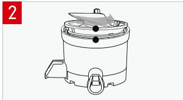
Twist the juicing screw down into the blank strainer.
