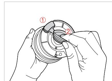
The silicon cover is removable for cleaning. After cleaning, insert the silicon cover as shown in the picture.
