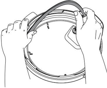
With the sealing ring removed, check the ring rack to make sure it is secured, centered, and an even height all the way around the lid. Do not attempt to repair a deformed ring rack.
