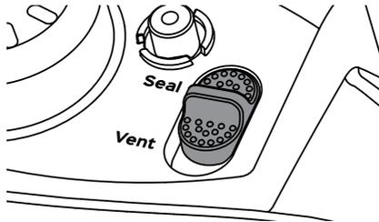
The quick release switch controls the steam release valve – the part that releases pressure.
