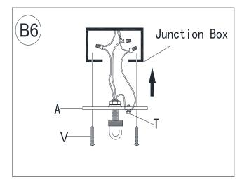
Attach the Mounting Plate (A) onto the junction box using two Mounting Screws (V).
