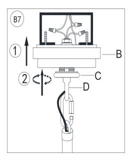
1. Slide the Canopy (B) upward along the Connection Tube (G) with the upper rim of the canopy pressed gently against the ceiling surface. Position the Canopy Nut (C) against the Fixture Loop (D) and rotate the nut clockwise to engage it with the threaded portion of the Fixture Loop (D) until secure. Do not over tighten this nut.
