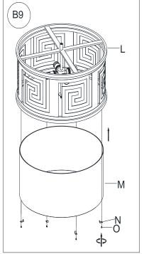
Attach Glass Shade (M) to Light Fixture (L) and secure by replacing Metal Tabs (N) to Light Fixture (L) and secure by tighten Screws (O).
