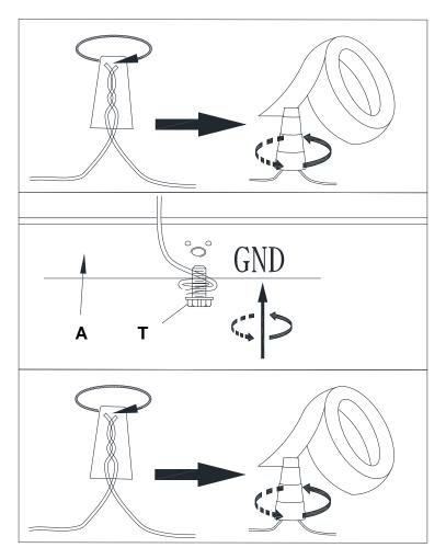
Connect the GROUND FIXTURE WIRE to the GROUND J-BOX WIRE using the Plastic Wire Nut Connector (U) and wrap the connection with electrical tape. Be sure that no wire strands are exposed.
