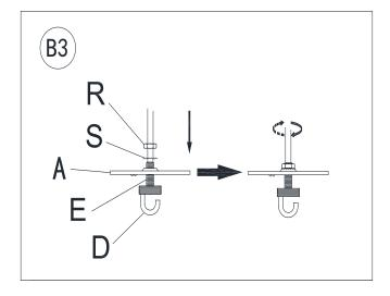
Position the Lock Washer (S) first and then the Hex Nut (R) onto the top end of Threaded Tube (E). Tighten the Hex Nut (M) until tight using pliers so that the Hanging Loop (D) is now firmly secured to the middle of the Mounting Plate (A).
