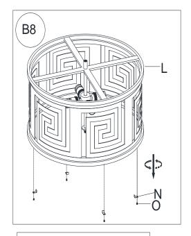
1. Remove Metal Tabs (N) from Light Fixture (L) by removing Screws (O).
