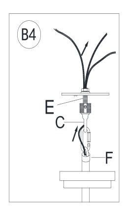
Feed the fixtures power cord and bare ground wire and Steel Cable through Hanging Loop (F) and Threaded Tube (E).
