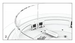
2. The round frameless glass installations are subject to tolerance and alignment issues. Please ensure that the glass screens have been properly pushed down into position and are not leaning outwards. If there are still alignment issues please adjust the screws where necessary with a Philips screw driver.
