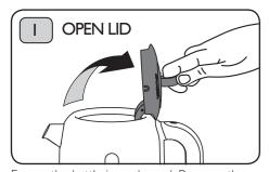
Ensure the kettle is unplugged. Remove the kettle from the power base. Gently pull the lid ring up and back to open the lid.
