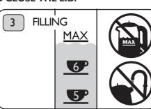
Fill the kettle through the lid opening. Use at least one cup of water (250ml). The water level must stay below the 'max' mark. Save energy, only boil what you require. Keep kettle upright and level at all times when filling. Do not tilt kettle backwards. **DO NOT OVERFILL OR**
