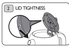
Tip: If the lid is too tight, try pushing in the pips on the inside of the lid with a spoon handle. Pushing the lid pips back out will give a tighter fit. WARNING: IF THE LID IS TOO LOOSE, RISK OF SCALDING.
