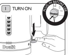
Plug the kettle into the power socket. Press the 'On/Off' switch down. The power neon will illuminate and the kettle will start to heat up. If the kettle is accidentally switched on with no water inside, the boil-dry device will switch off the Always unplug the kettle after each use. heating element to prevent damage to the kettle.
