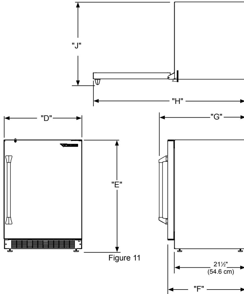
\* Depth dimension of rough-in opening may vary depending on each individual installation. To recess entire door "F" dimension plus 1" (2.5 cm) for thickness of power cord plug is required.
