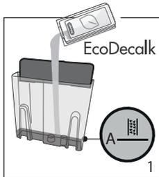
1. (IF PRESENT, REMOVE THE WATER SOFTENER DEVICE). Pour the descaler into the tank up to the level A marked inside the tank (equal to one 100ml packet).
