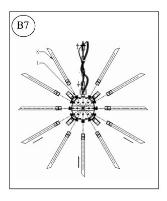
Insert the Glass Rods (K) onto the Jointing Ends (L) that located around the fixture ball. Make sure each glass rod is inserted into place so the small pin on the Jointing End (L) clicks & locks the glass rod securely.
