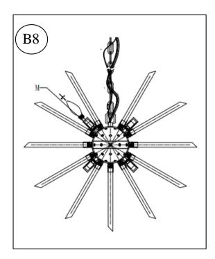
Insert the specified light bulbs into the Sockets (M). DO NOT EXCEED THE SPECIFIED WATTAGE.
