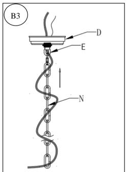
Weave the fixtures 2 wire power cord and bare ground wire through every other loop to the top of Chain (N), and then through the Hanging Loop (E) and Canopy (D).
