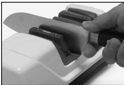
Figure 17. Insert your index finger as shown behind the choil as the knife is inserted into the sharpening slot (see Suggestion 8.)
