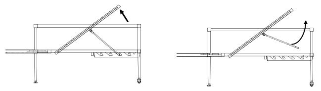
2) Place the stay bar flat towards the end of the head; **DO NOT** place the end of back.
