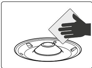
Keep the pan sensor clean, dry and free from oil build-up on and around sensor.
