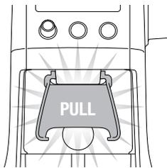
Slide in grinds container with cap open or coffee filter directly under grind outlet.
