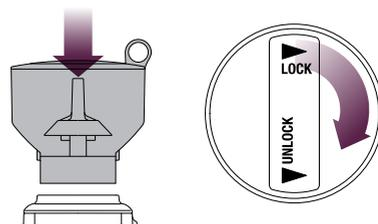
The bean hopper can be removed by turning dial anti clockwise and lifting hopper to pull out. The locking system allows you to remove and transfer beans in the hopper to a storage container safely.
