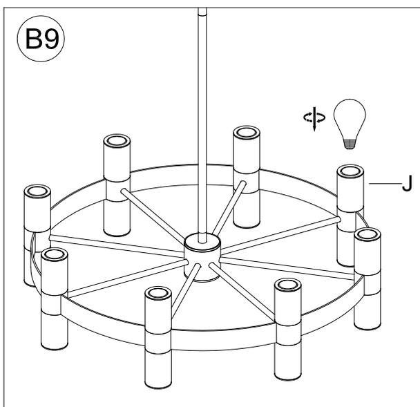
Insert eight (8) **40-watt maximum TYPE A standard incandescent light bulbs** (not included) or eight (8) **9-watt compact fluorescent light bulbs** (not included) into the Sockets (J). **DO NOT EXCEED THE SPECIFIED WATTAGE.**
