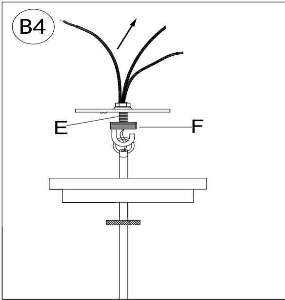
Feed the fixtures power cord and bare ground wire and Steel Cable through Hanging Loop (F) and Threaded Tube (E).
