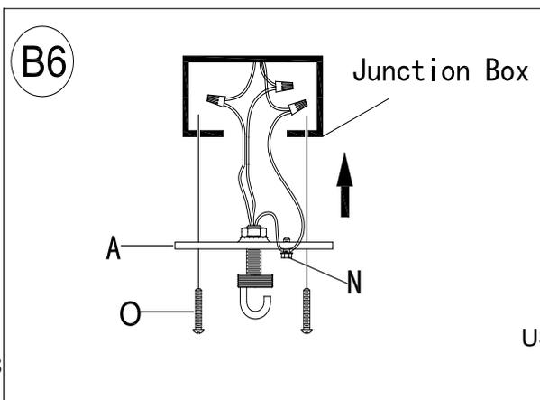
Attach the Mounting Plate (A) onto the junction box using two Mounting Screws (O).
