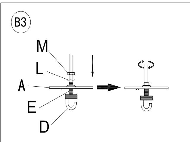
1. Position the Lock Washer (L) first and then the Hex Nut (M) onto the top end of Threaded Tube (E). Tighten the Hex Nut (M) until tight using pliers so that the Hanging Loop (D) is now firmly secured to the middle of the Mounting Plate (A).
