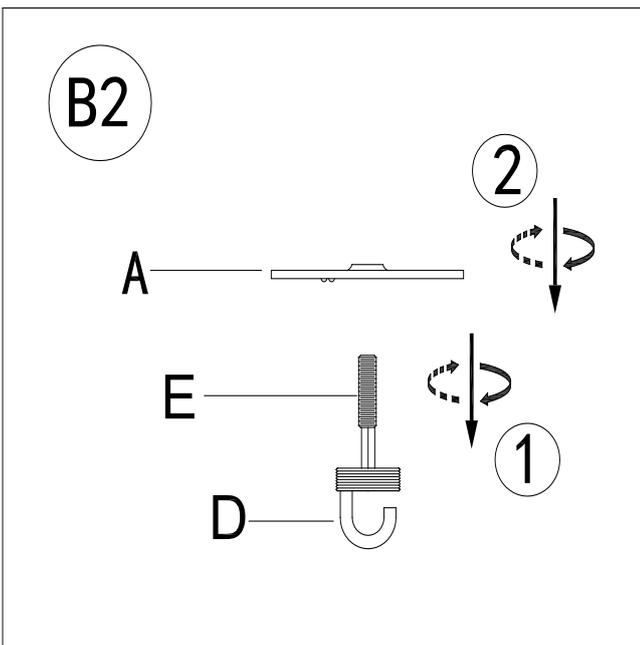
1. Attach the Threaded Tube (E) into the threaded bore of the Hanging Loop (D) and rotate the Threaded Tube (E) clockwise until it is tightly engaged within the Hanging Loop (D).
