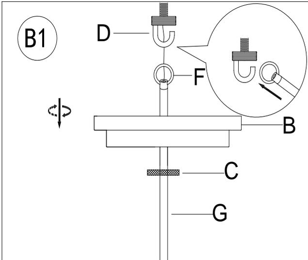
1. Hook the Hanging Loop (F) onto the Fixture Loop (D).
