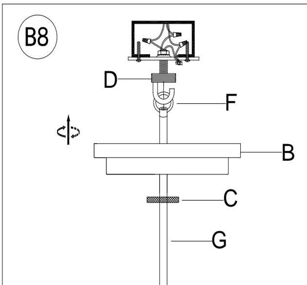
Slide the Canopy (B) upward along the Connection Rod (G) with the upper rim of the canopy pressed gently against the ceiling surface. Position the Canopy Nut (C) against the Hanging Loop (D) and rotate the nut clockwise to engage it with the threaded portion of the Hanging Loop (D) until secure. Do not over tighten this nut
