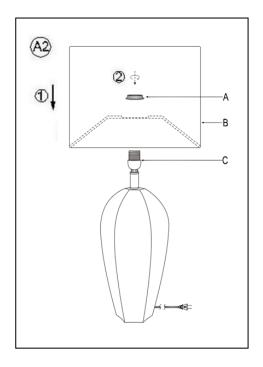
Place the Shade (B) over onto the Socket (C) and secure the shade in place by turning the Socket Ring (A) in a clockwise direction until tight.
