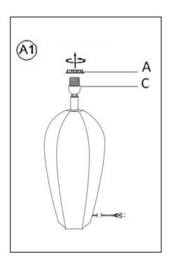
Unscrew Socket Ring (A) from Socket (C) by turning counter-clockwise.
