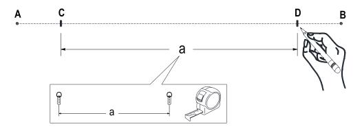
Use a stud-finder to determine if there is a wall stud[s] located at [each] either insertion mark.
