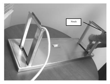
Install the RIGHT Pass Shelf Bracket, in the same manner, assuring that the open notch on the upper portion of the bracket is facing toward YOU. Use (2) 1/4-20 x 3/8 Phillips Truss Head screws to secure.
