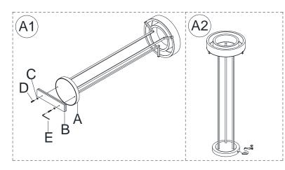
Remove Legs (B) from Fixture Base (A) by removing Metal Disk (C) and bolts (D) with Wrench (E). (Refer to A1)
