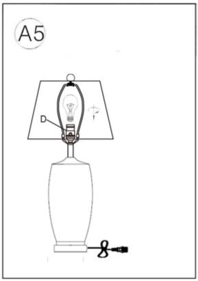
Insert the specified light bulb into the Socket (D). DO NOT EXCEED THE SPECIFIED WATTAGE.
