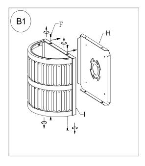
Separate the Mounting Plate (H) from the Metal Base (I) by removing the 4 Canopy Screws (F). Do not discard the Canopy Screws (F) as these will be used later.
