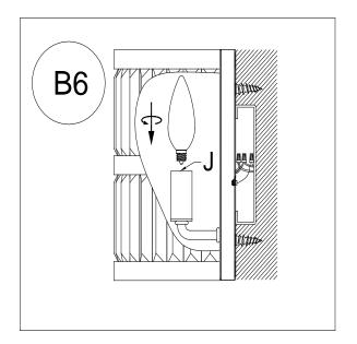
Insert the specified light bulbs into the Sockets (J). DO NOT EXCEED THE SPECIFIED WATTAGE.
