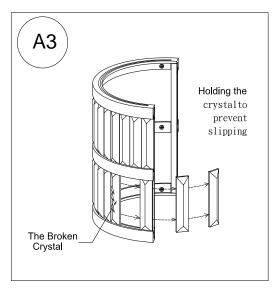
Place the light fixture on a work place; carefully hold the crystal to prevent to slip. Take out the broken crystal
