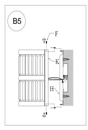
Attach Light fixture (K) to the affixed Mounting Plate (H), align the holes and secure with Canopy Screws (F).
