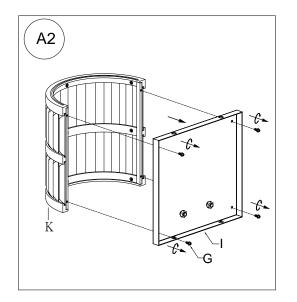
Separate the Metal Base (I) from the Light Fixture (K) by removing the 4 Screws (G). Do not discard the Canopy Screws (G) as these will be used later.
