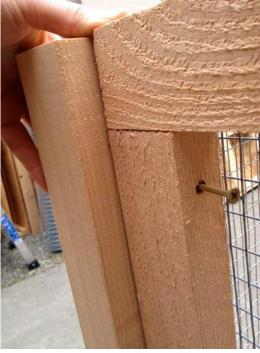
5. After the three frames are screwed together, square them up and install the door frame. The door needs to be opened to access the pre-drilled holes (see picture below). The screws are provided in the fastener and hardware bag that it shipped inside the planter box. The frame should be set 1" in from the face of the posts as well. Assemble this last frame and close the door (you can carefully hold up the in the open position by propping it up under a 3" block of wood.
