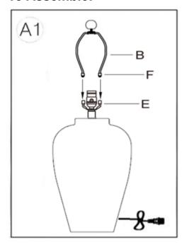
Raise the Harp Caps (F) and insert the bottom ends of Harp (B) into the Saddle (E)  $\,$
