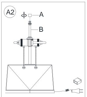
2. Remove Finial (A) from top of Rod (B) by turning counter clockwise direction.
