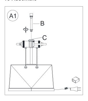
Thread Rod (B) into the center opening of Middle Box (C) by turning clockwise direction until tight.
