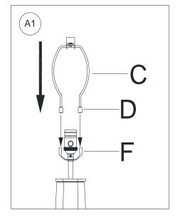
Raise the Harp Caps (D) and insert the bottom ends of Harp (C) into the Saddle (F)
