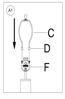
Raise the Harp Caps (D) and insert the bottom ends of Harp (C) into the Saddle (F)
